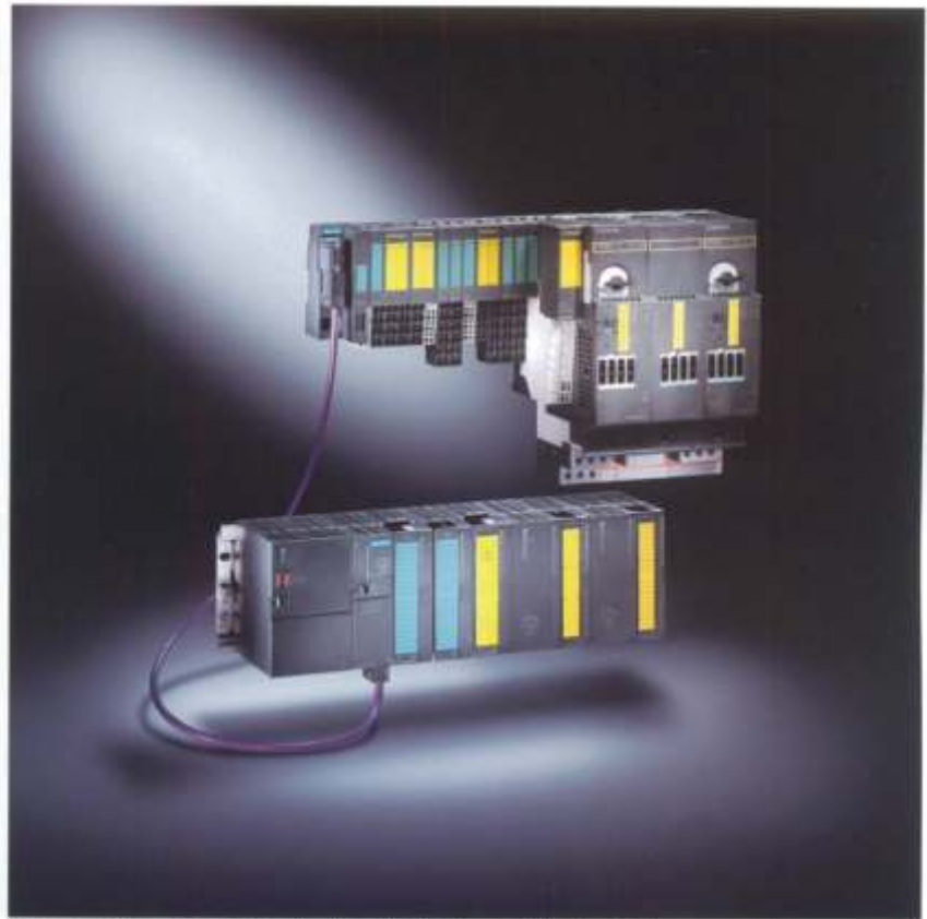
Mixed configuration of standard and fail-safe modules, including motor starters
